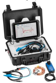
The IRG 400 time domain reflectometer in the portable case version with removable tablet. (Pictures: BAUR GmbH)
